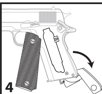
2. Remove left grip cover by lifting at the bottom of the grip. Flip up puncture lever as shown. (Fig. 3)
